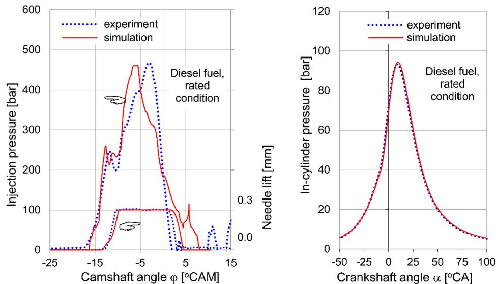
**Figure 3 Injection pressure, needle lift, and in-cylinder pressure at full load**
