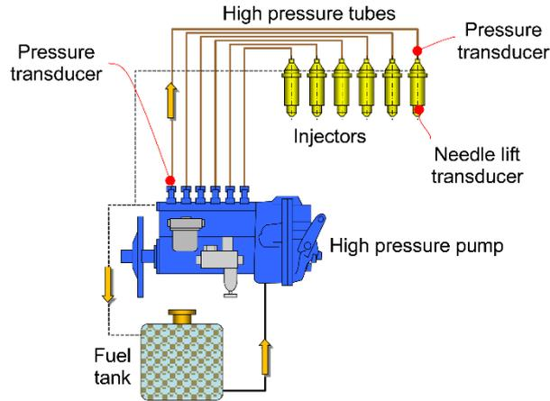
**Figure 1. The fuel injection system test bed**
