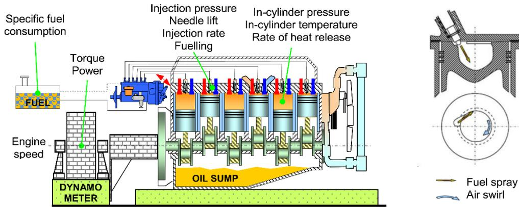
**Figure 2 The bus diesel engine test bed**
