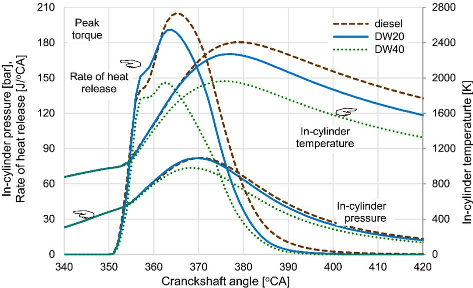
**Figure 8 Combustion characteristics at peak torque condition**
