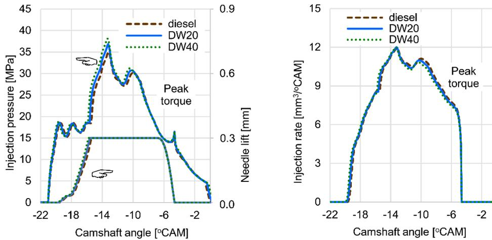
**Figure 4 Injection characteristics at peak torque**
