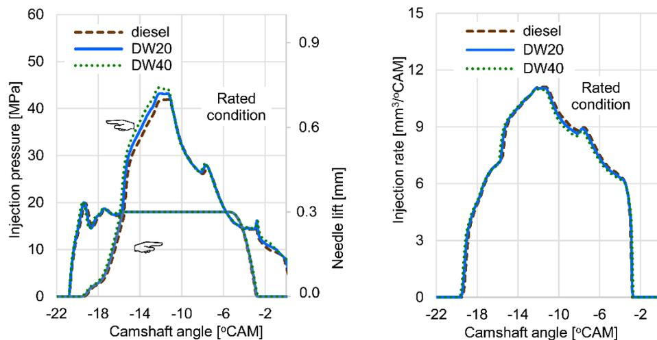
**Figure 5 Injection characteristics at rated conditions**
