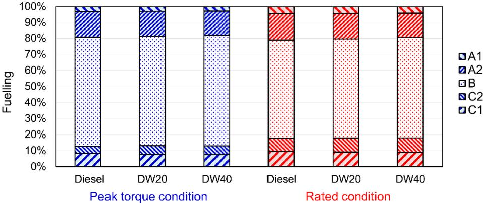
**Figure 6 Fuelling in different phases of injection**
