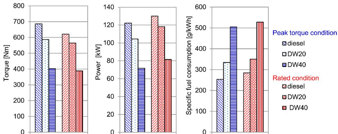
**Figure 10 Engine characteristics at peak torque and rated condition**
