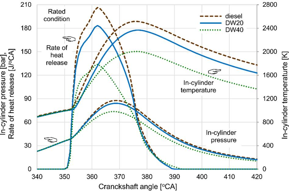
**Figure 9 Combustion characteristics at rated condition**
